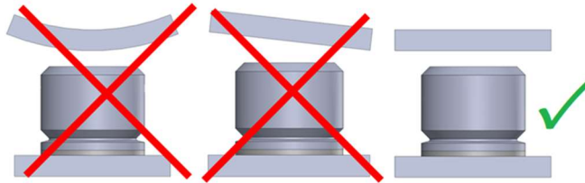
Fig. 4: counter-pressure plates even and parallel moving
